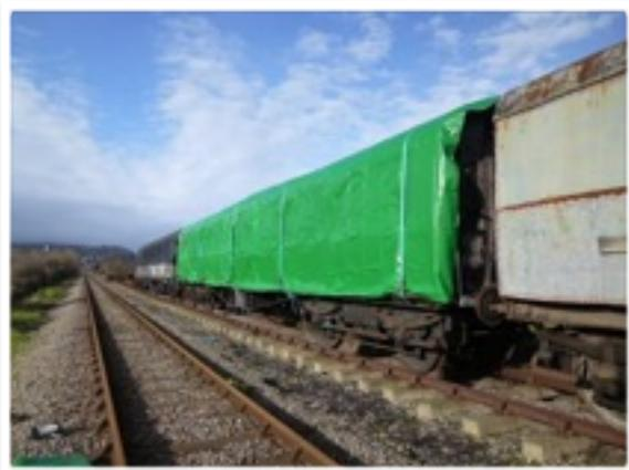
The plastic sheeting on some of the coaches at Williton is not standing up well to the wind either, and quickly deteriorates because of the UV rays from the sun (when we see it). What the wind doesn't damage, the
