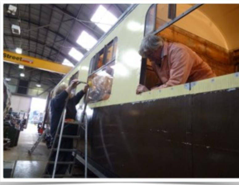
Work has also started on stripping the paintwork which has to be renewed as a consequence of replacing the windows, and because some of the first application of paint had started to peel off. A different technique will be used to ensure an immaculate finish for the completed coach in the best Swindon tradition.
