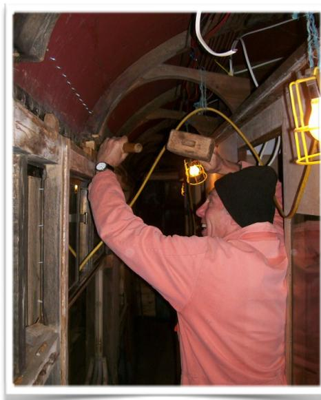
The other requirement to complete the body of the vehicle is to fit the gangway connections. The frames for these have been cleaned and painted and can now go to the South Devon Railway at Buckfastleigh to have the bellows and wire hoops fitted.
