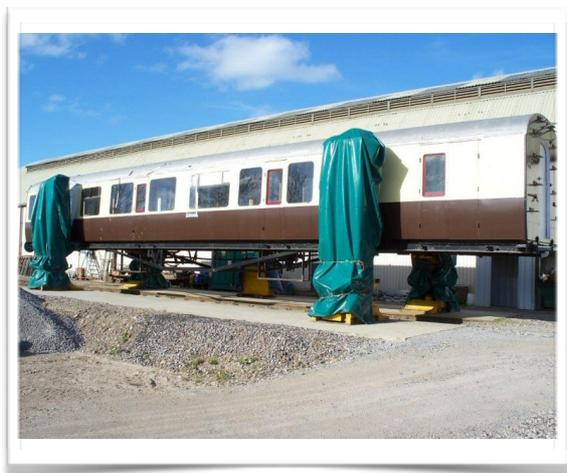
During the summer, the coach was lifted and the bogies removed, stripped down, cleaned and repainted. Worn and broken components have been replaced (the eye bolts are being machined at Williton currently for fitting before the end of the year). While it was on jacks, the opportunity was taken to complete painting of the underframe and to treat the wooden floor of the coach with wood preservative.
